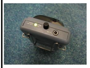
The indicated light will be on when turn on the transmitter. Turn the black button to adjust the volume.
