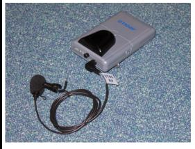
Connect the Tie-clip Microphone to the Transmitter.
